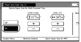
**6** Press [On] and press [+] or [–] to set the Y (Length) and X (Width) sizes.
